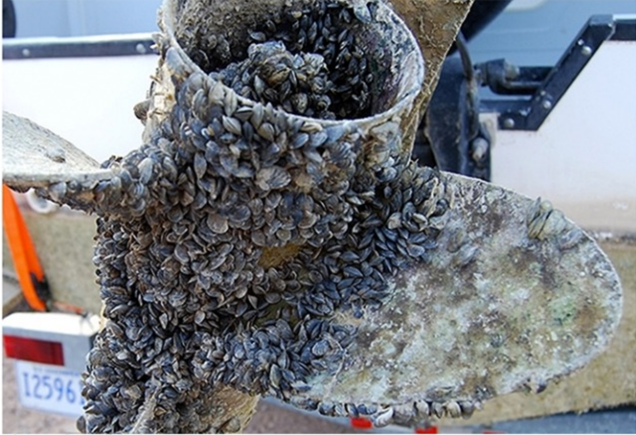
A boat propeller engulfed with quagga mussels. Image Credit: US National Parks Service
